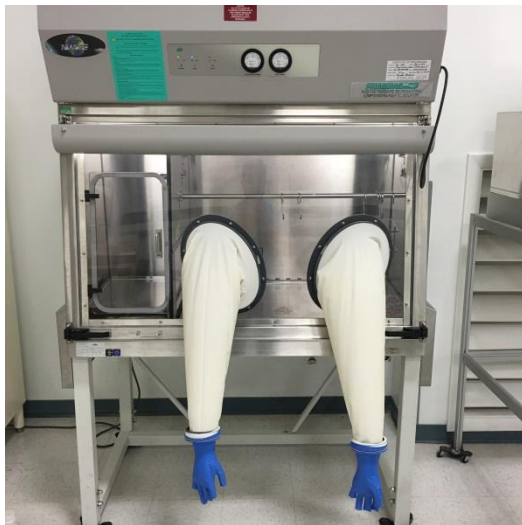
Nuare Pharmagard Positive Pressure Recirculating Compounding Aseptic Isolator with HEPA filtration.
