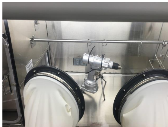
Nuare Pharmagard Positive Pressure Recirculating Compounding Aseptic Isolator with HEPA filtration.
